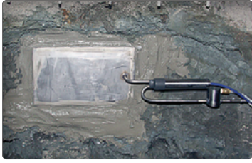
● Model 4850 NATM Shotcrete Stress Cell with remote re-pressurization option.
